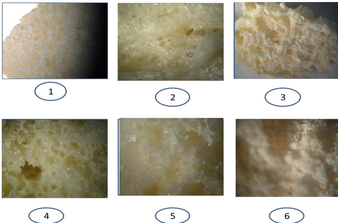
Figure 13: Optical micrograph of the polyurethane scaffolds hydrolytic degradation
