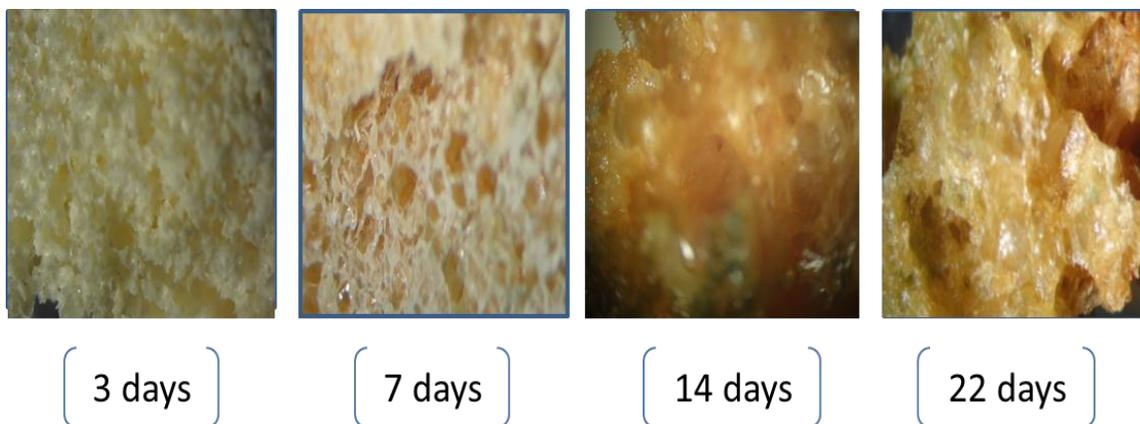
**Figure 15: Optical micrograph of polyurethane scaffolds during oxidative degradation**
