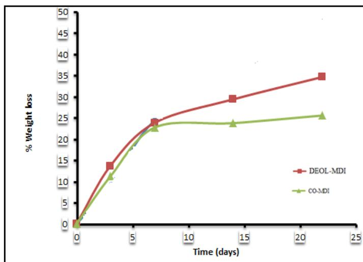
Figure 14: Mass loss of polyurethane scaffolds during oxidative degradation in 37 C °
